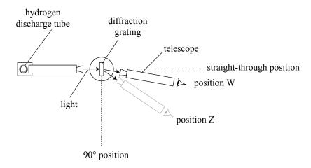
As the telescope is rotated from W to Z, each of the 4 lines of the first order spectrum is seen in turn.
